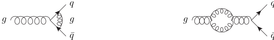
Figure 7: Example virtual corrections contributing to the evolution of the strong coupling constant.
